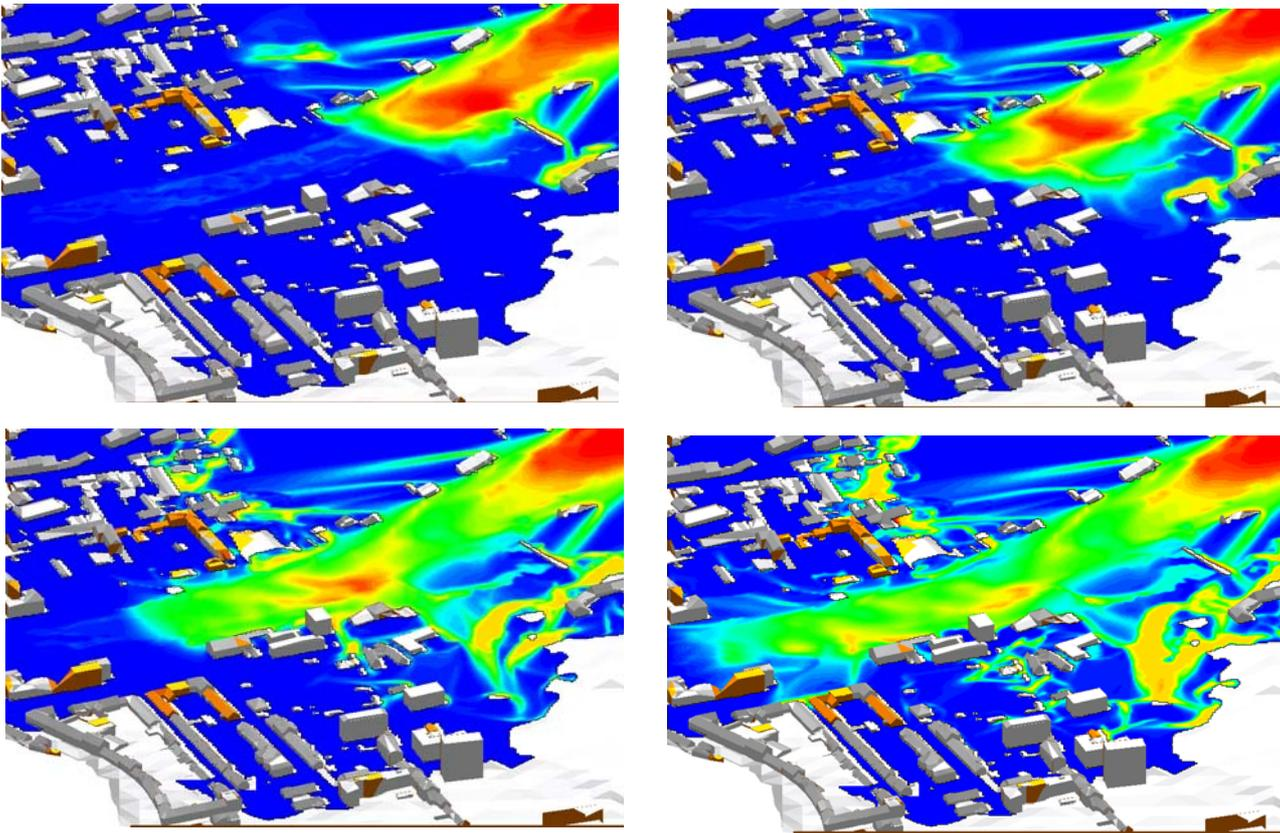
Figure 2: Computed volume fraction of the water during the flood phase
